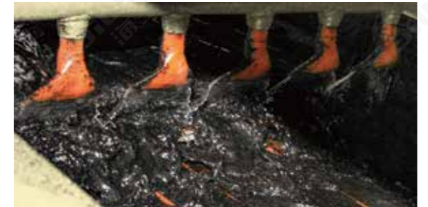
Motion and material status during the actual classifying process of multi-layer screen
