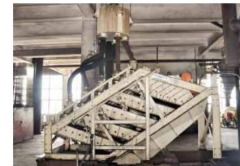
On-site shooting of laminated vibrating screen application
