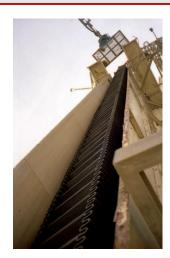
In inclined transport with germanBelt® corrugated sidewall conveyor belts we use laterally stable conveyor belts - the germanCross basic belts. This lateral stability makes it possible to change horizontal to vertical direction of travel to vertical and vice versa.
