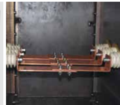
Test setup for arcing fault test with up to 66 kA
