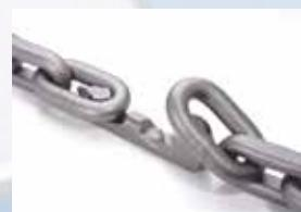
2. Lay chain ends into one connector half
