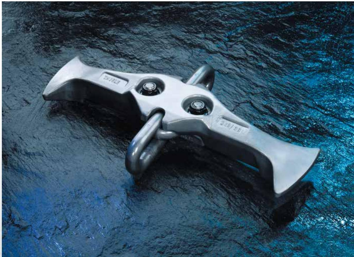
THIELE Single Strand Flight Bars are designed for single-strand chain conveyors. The accurately forged and calibrated chain recess ensures a smooth chain run and prevents the flight bar from wandering out of the pan profile.
