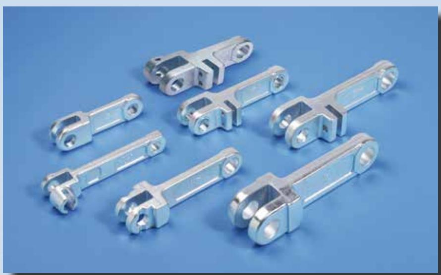
THIELE manufactures forged link chains as complete assemblies and the company's in-house forging plant has access to a wide range of dies – which means that THIELE can supply a broad spectrum of designs for all commonly used chain pitches of 100 - 300 mm.
